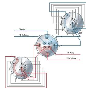
Schematic overview of a multiple heart-cut valve setup [3].
